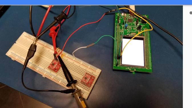
STMicro Discovery board hooked up to a SparkFun IMU breakout board to test I2C communications
